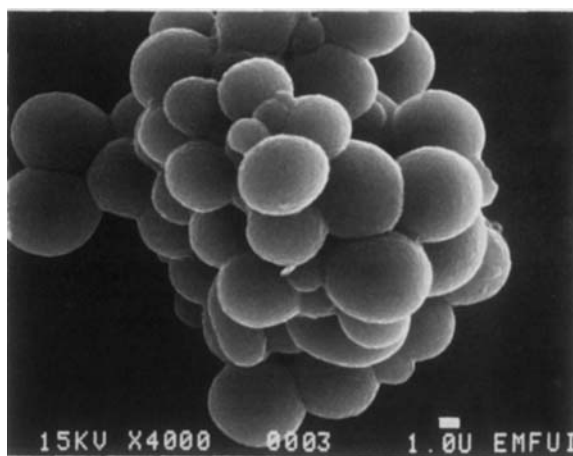
FIG. 1. Scanning electron micrograph of albumin/acacia coacervate particles prepared at pH 4.2 and stored at 40°C for forty-six days.
